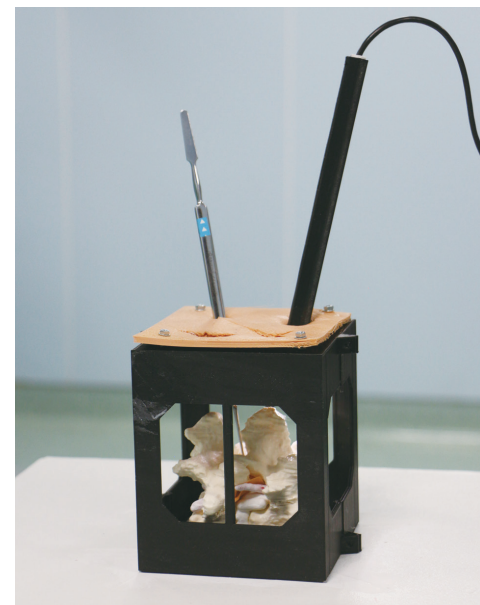
Fig. 3. Assembled version of the model. A black cardboard wrap held with long tail clips was used in our study to force the trainee to use the endoscopic view, but surgical sheets may also be used.
